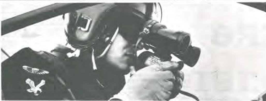
Soldier using gyroscopically stabilised binoculars for surveillance
